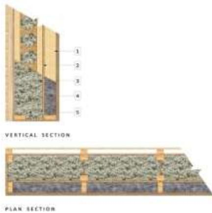
The ECO-SEE external wall panel is made up of a specially developed timber frame, which incorporates ECO-SEE insulation and internal coatings. The panel has been developed to improve the indoor air and environment quality of buildings through the use of materials that capture VOCs and regulate humidity.
