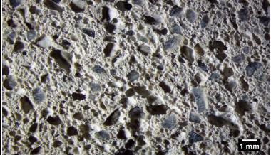
Aerogel Foam Concrete is a composite inorganic insulation material that brings together the advantages of foam concrete in terms of workability and sustainability (low embodied energy) with the thermal insulation capacity of the aerogels. The material is suitable for application in lightweight sandwich facade elements for new buildings and renovation and for indoor partition walls. The material is developed by **Aercrete Technology AB** in collaboration with **Svenska Aerogel AB**.
