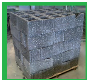
GEO blocks made of SUS-CON concrete ( \lambda=0.155 W/mK)
