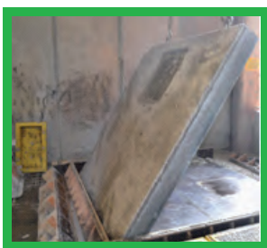
GEO panels made of SUS-CON concrete ( \lambda=0.165 W/mK)
