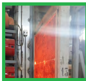
Fire resistance tests on GEO panel (EI240)
