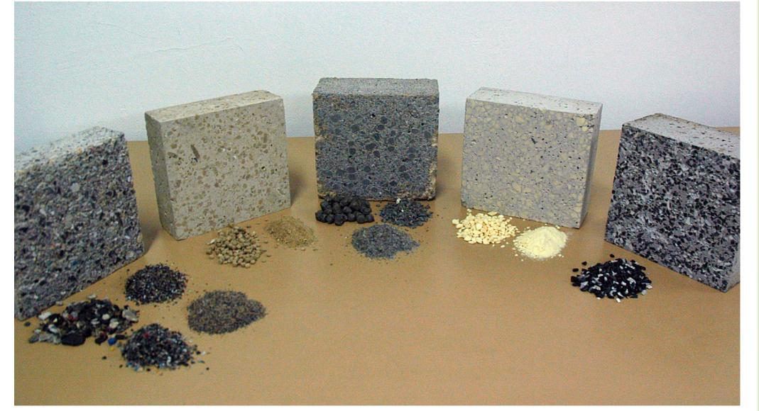
Development of a new generation of inorganic insulation materials andbuilding insulation masonry components ("3I") with lower embodied energy (50% reduction), lower cost (cheaper by 15%) and upgraded properties compared to current technology.
